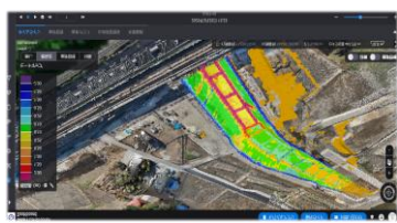
Automatic management of earth volume through ICT earthwork
